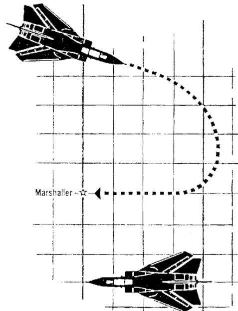
If obstructions exist, two extra personnel may be required to complete the marshalling team. They would walk on either side of the aircraft, ahead of the wing tips and signal to the pilot if there is sufficient clearance for the aircraft to pass the obstructions. This assistance is most likely to be necessary when marshalling large aircraft with restricted fields of view from the cockpit.
